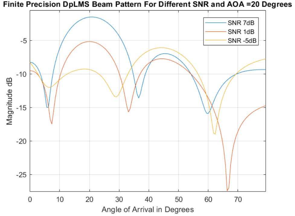
Figure 5.12 – Finite Precision DpLMS Beam Pattern for Different SNR
