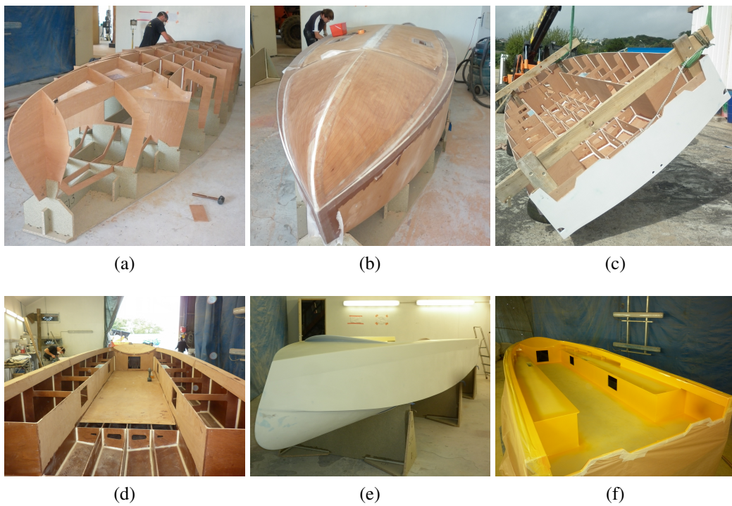
Figure 6.3.: Pictures of construction steps of the kiteboat.
