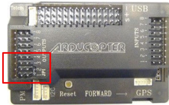
Figure 5.5: Arduino output pins for ESCs
