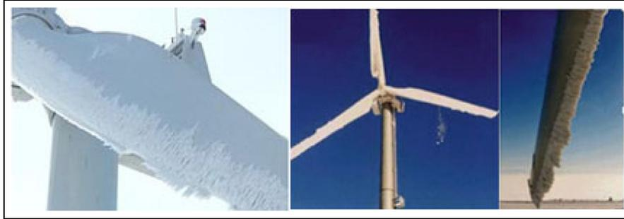
**Figure 1.** Impact of icing on wind turbines.
