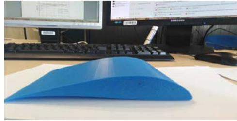
(c) Hydrofoil Manufacture using Additive Manufacturing
