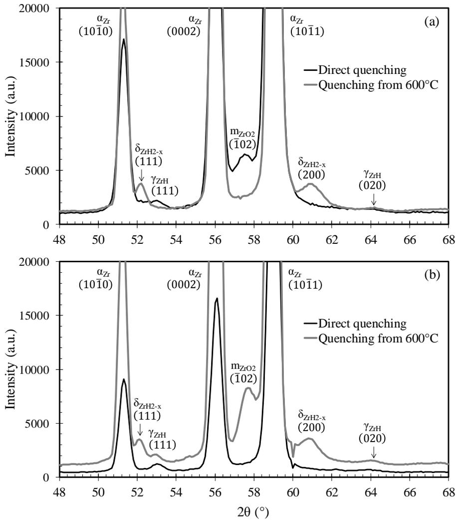
**Fig. 12.** Neutron diffraction patterns recorded at RT on (a) Zircaloy-4 and (b) M5 containing about 320 wppm of hydrogen after water quenching from 1000°C or cooling at 0.4-1°C/s from 1000°C down to 600°C then water quenching.
