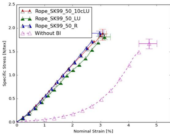
Figure 12. c. Rope results for a maximal BI load of 50% of the MBL.
