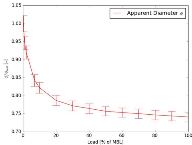
Figure 17. Change in the apparent diameter with tension loading. Error bars show standard deviation.
