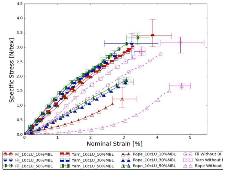
Figure 13.f. Tension after 10 load/unload cycles BI
