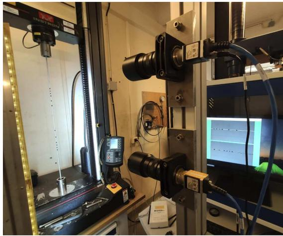
Figure 4. Monotonous loading on rope with different markers
