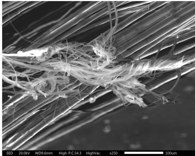
Figure 15. SEM image of extracted Dyneema filaments
