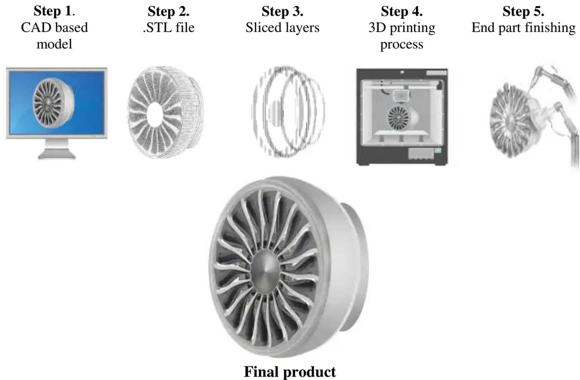
Figure 1: 3D printing process flow (Graphic: Deloitte University Press).
