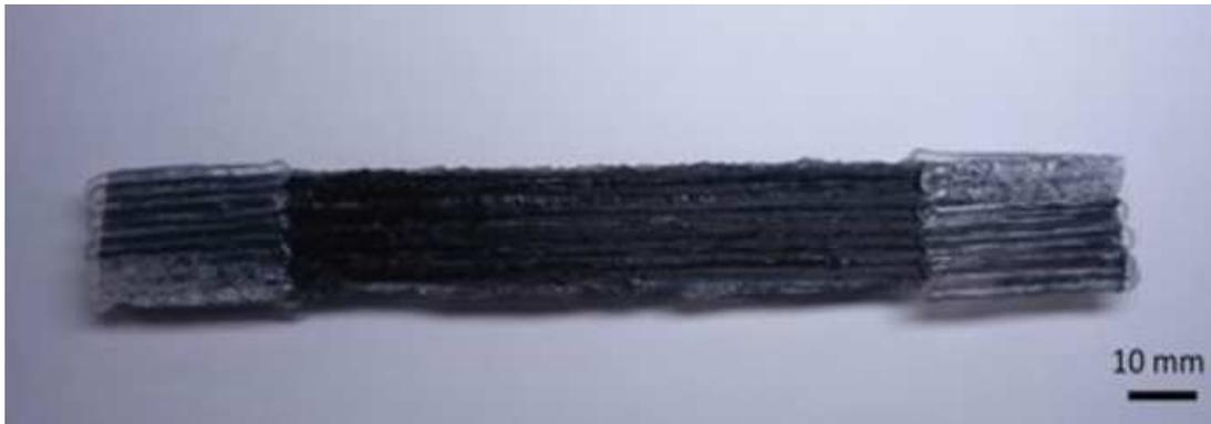
Figure 13: Example of 3D printed UD fiber composites [133].
