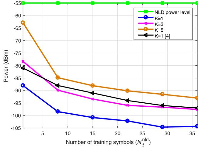
**FIGURE 4** The power of the residual nonlinear distortion (NLD) in terms of the number of training symbols for different values of the NLD order. The received signal power is fixed to 0 dBm and the NLD power is  $-56$  dBc (ie,  $-56$  dBm for a 0-dB gain of the low-noise amplifier)
