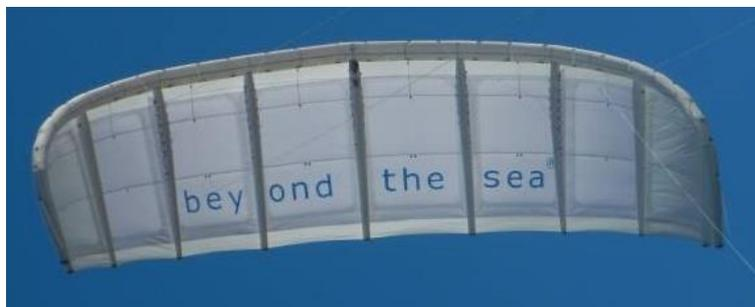
Fig. 1: Kite used during measurement. C-shape with inflatable leading edge and battens, 50m<sup>2</sup>, 23 kg (deflated, with bridles and tethers).
