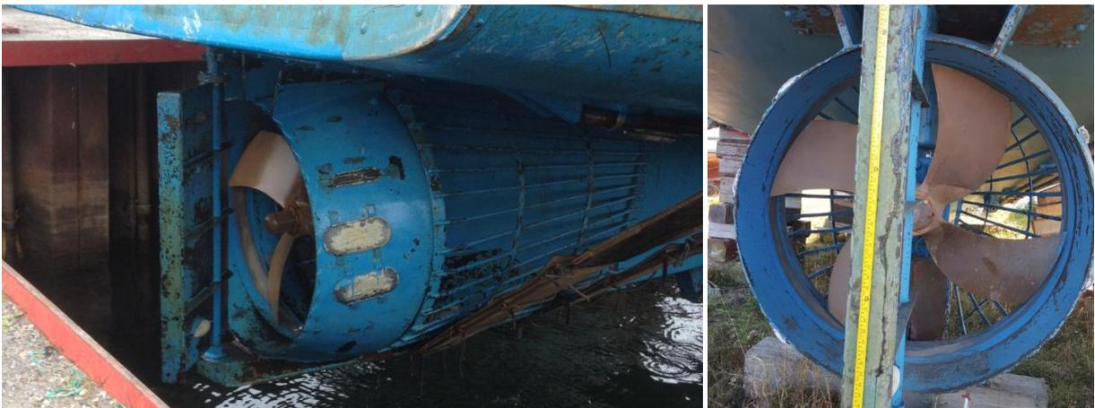
Fig. 5: Pictures of the Steven Paul propeller and rudder.
