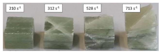
Fig. 11. Recovered specimens after IP dynamic compression tests.
