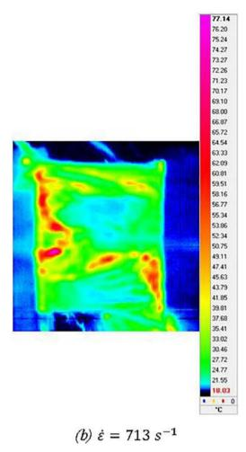
Fig. 13. Heating of the sample during damage.
