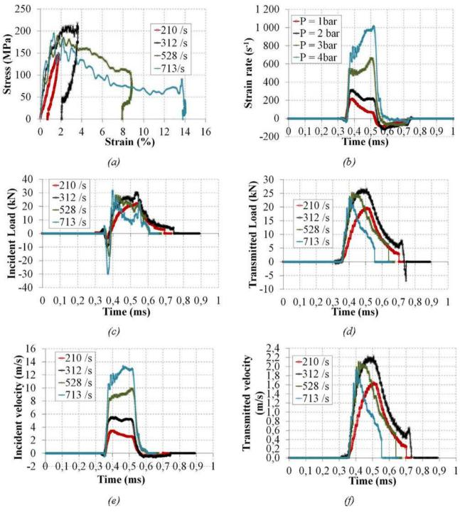
Fig. 7. Dynamic parameters for different impact pressures.
