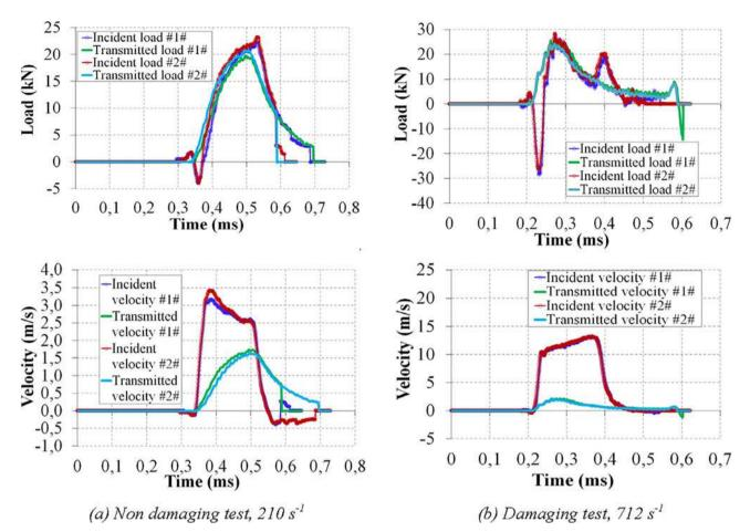
Fig. 6. Test reproducibility for IP tests, Incident and transmitted loads and velocities.
