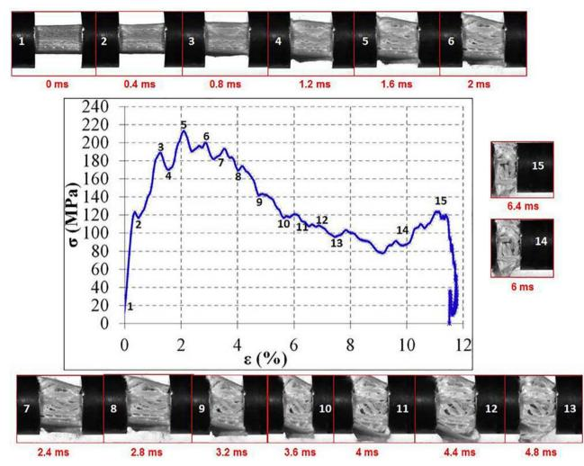
Fig. 12. High speed photograph of real-time dynamic compression test of adhesively bonded joints impacted at high strain rate of 713 s<sup>-1</sup>.
