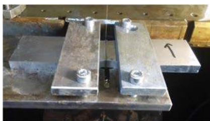
Fig. 16 Part clamping during wire electro-discharge machine cutting
