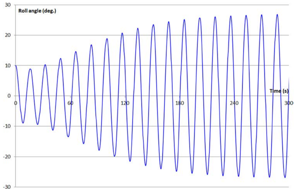
Fig. 2 Roll angle versus time in parametric resonance condition
