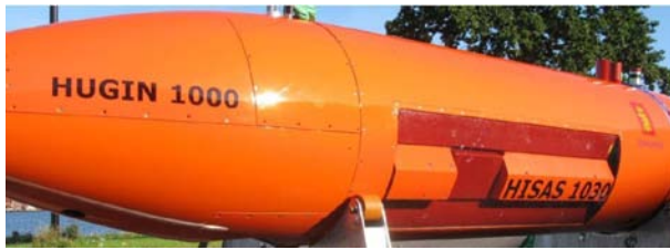
Fig. 2. The HISAS 1030 interferometric SAS mounted on a HUGIN autonomous underwater vehicle.
