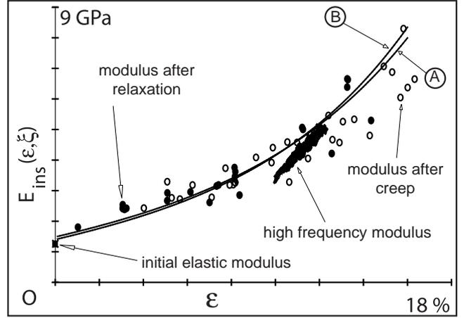
Figure 28: Instantaneous modulus in monotonous and cyclic loading for the three groups of straps compared to curves A and B computed by relation 22 and material parameters of table 2.
