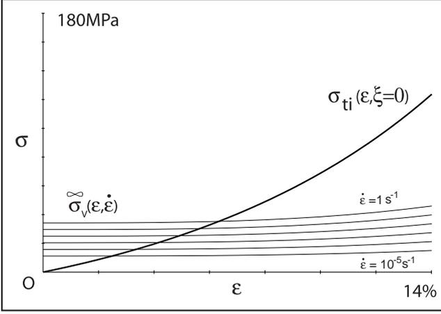
Figure 33: Steady state viscous stress  $\sigma_v^\infty(\varepsilon, \dot{\varepsilon})$  (thin line) and time-independent stress  $\sigma_{ti}(\varepsilon, \xi = 0)$  (bold line) for the group *A* straps.
