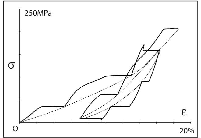
Figure 30: Estimated time-independent behaviour (dashed line) based on the state at the ends of the creep periods of test A36 (fig. 17).
