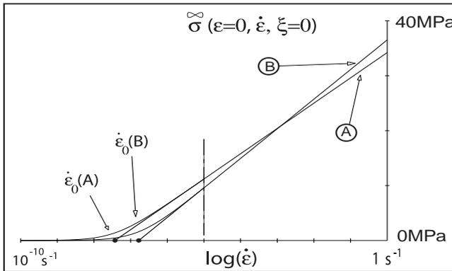
Figure 23: Steady state stress at a strain equal to zero and in monotonous tensile. Signification of parameter  $\dot{\varepsilon}_0$  of relation 8.
