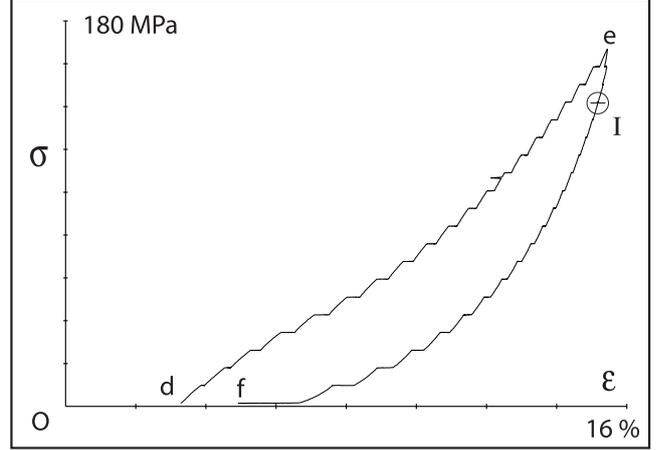
Figure 39: Result of test *A40b* controlled at constant stress rate ( $\dot{\sigma} = 1,3 \text{ MPa/s}$ ) and broken by a lot of creep periods of very short duration (15s).
