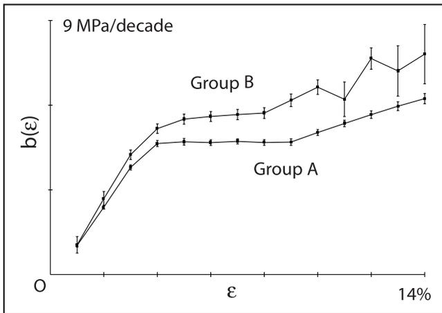
Figure 13:  $b(\varepsilon)$  parameter as result of the linear regression, computed on the data of strap groups A and B. Above and below each point  $b(\varepsilon)$  are shown the values of standard deviation.
