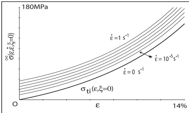
Figure 25: The steady state stress  $\tilde{\sigma}(\varepsilon, \dot{\varepsilon}, \xi = 0)$  (thin line) and the time-independent stress  $\sigma_{ti}(\varepsilon, \xi = 0)$  (bold line) for the group B straps.
