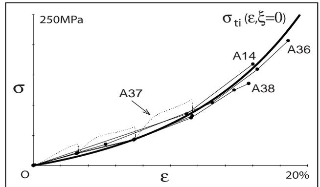
Figure 26: Comparison of the time-independent stress  $\sigma_{ti}(\varepsilon, \xi = 0)$  computed by relation 16 and material parameters of table 2 (bold line) and the stress at the ends of relaxation and creep stages (thin line and bold points).
