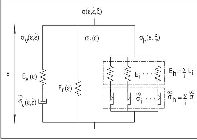
Figure 3: Visco-elasto-hysteresis behaviour model in the one-dimensional case.
