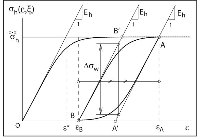
Figure 31: Time-independent stress  $\sigma_{ti}(\varepsilon, \xi)$  measured by means of relaxation test A38 and creep test A36. Figure 32: Method of measurement of the yield stress  $\sigma_h^\infty$  of the pure hysteresis component.
