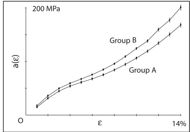
Figure 12:  $a(\varepsilon)$  parameter as result of the linear regression, computed on the data of strap groups A and B. Above and below each point  $a(\varepsilon)$  are shown the values of standard deviation.
