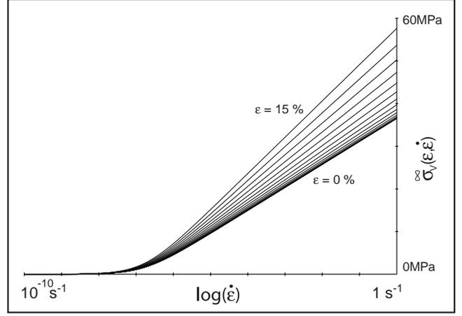
Figure 34: Steady state viscous stress  $\sigma_v^\infty(\varepsilon, \dot{\varepsilon})$  as a function of the strain rate at different strains for the group *B* straps.
