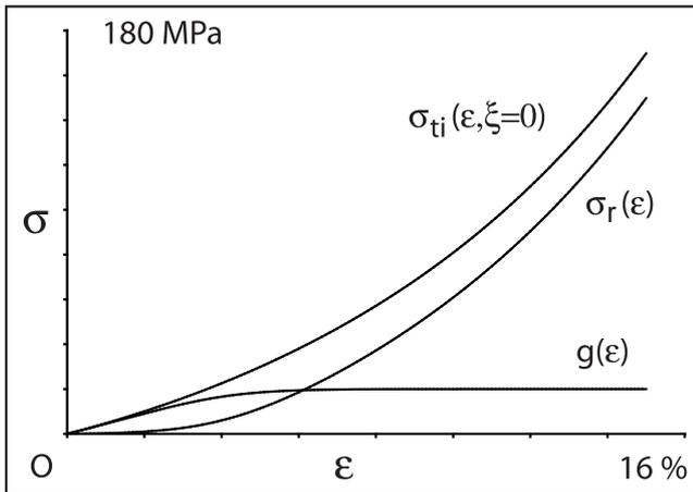
Figure 36: Time-independent stress  $\sigma_{ti}(\varepsilon, \xi = 0)$  in monotonous loading and its splitting up into reversible stress  $\sigma_r(\varepsilon)$  and pure hysteresis stress  $g(\varepsilon)$  in monotonous loading, for the group B of straps.
