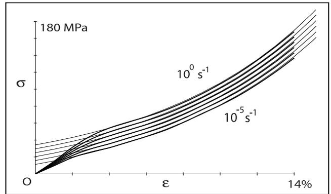
Figure 24: Stress in monotonous tensile  $\sigma(\varepsilon, \dot{\varepsilon}, \xi = 0)$  (bold line) and related steady state stress  $\tilde{\sigma}(\varepsilon, \dot{\varepsilon}, \xi = 0)$  (thin line) in the case of the group A straps.
