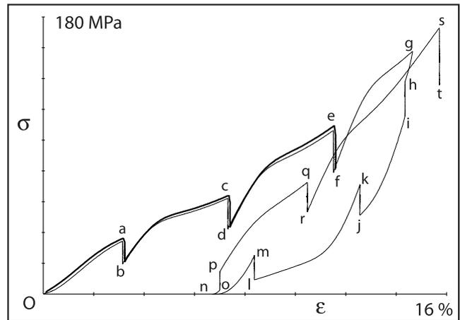
Figure 14: Results of two cyclic tensile tests with relaxation periods ( $\dot{\varepsilon} = 10^{-3} \text{ s}^{-1}$ ); A37 (bold line) and A38 (thin line).
